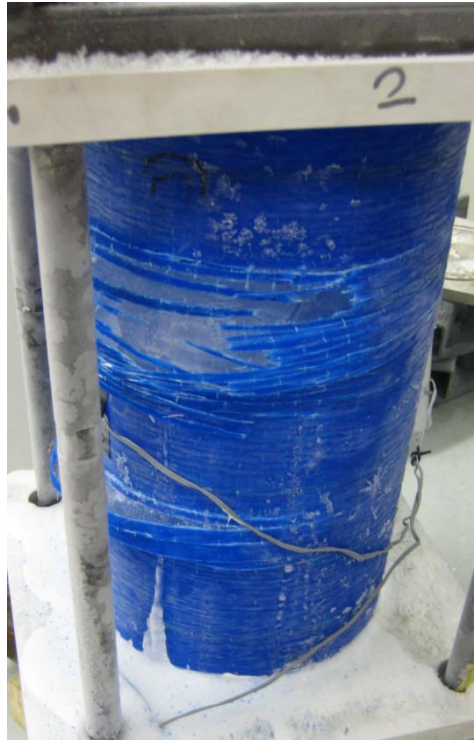
Figure 40 – Typical tensile failure observed on specimen 1P-171-2.
